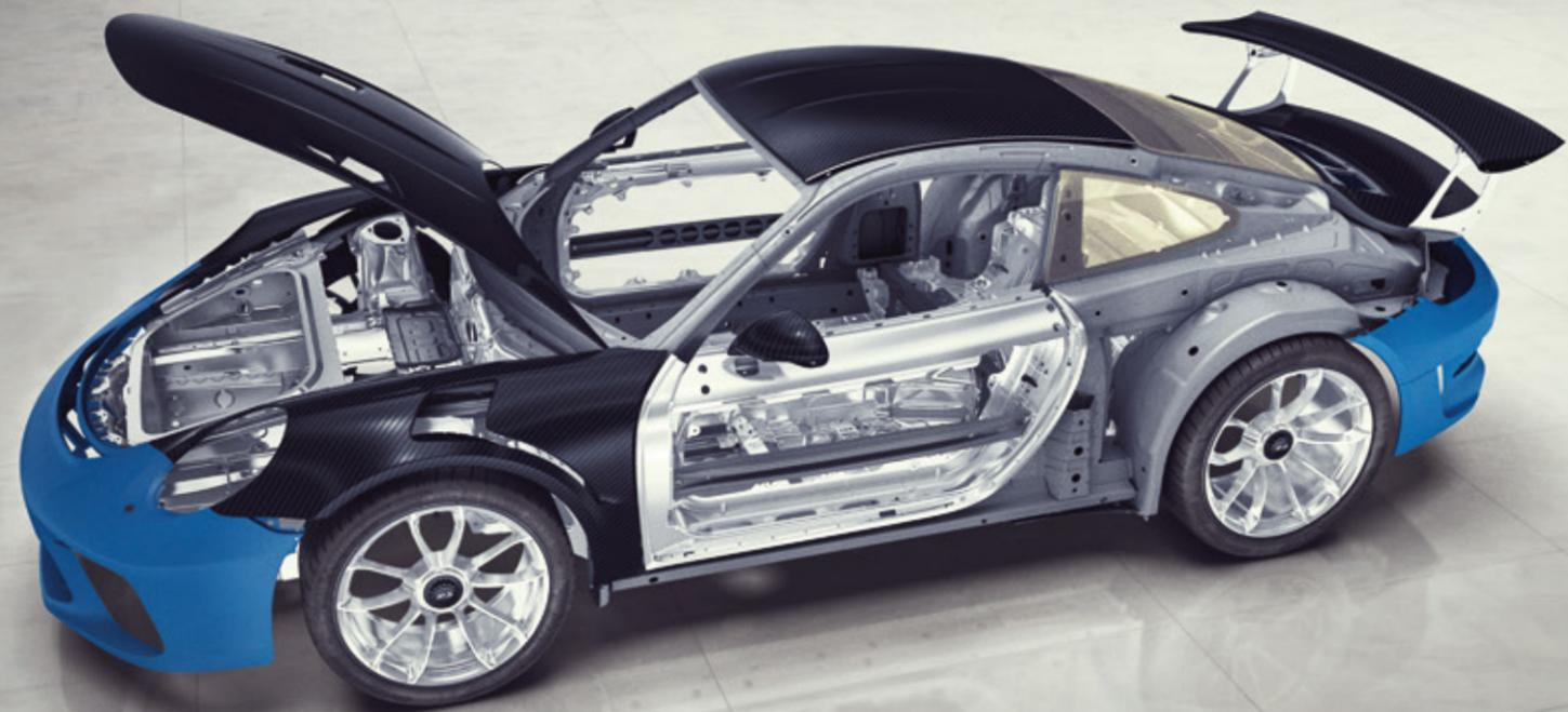
■ Carbon-fiber reinforced plastic (CFRP)   ■ Lightweight polyurethane   ■ Aluminum   ■ Lightweight glass
