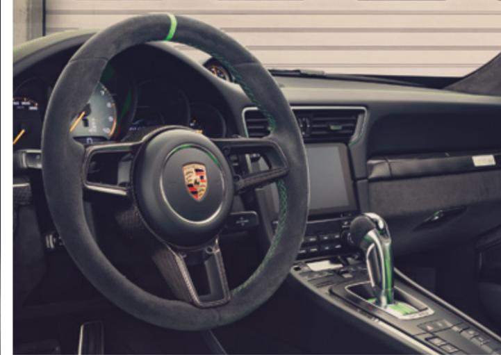
Every gram counts, and so does every detail. For this reason, the ultra-light gearshift paddles and the steering wheel trim are in carbon-fiber reinforced plastic (CFRP) with a carbon-weave finish. In their search for further weight savings, our vehicle developers have even made the carpet trim lighter.
